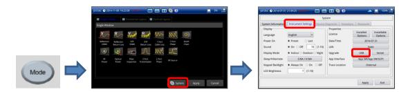
Select your downloaded firmware file from the list box by using the Up/Down Arrow keys or the rotary knob to navigate until you find the latest version KKC\_FW\_1.054.001.FW.
