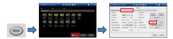
Select your downloaded firmware file from the list box by using the Up/Down Arrow keys or the rotary knob to navigate until you find the latest version KKC\_FW\_1.051.015.FW.
